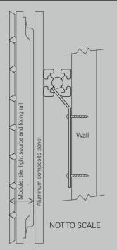
This is a conceptual drawing showing a cross section, side view of the mounting hardware which is connected to the backside of the light surface and secured into the wall bracket.
